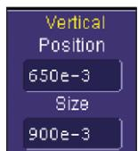
There are no dedicated front panel controls for digital line position and size. However, you can touch the controls (shown at left) twice and enter in a unitless value for position and size using the pop up keypad or you can touch them once and use the front panel adjustment knob to adjust the value.
